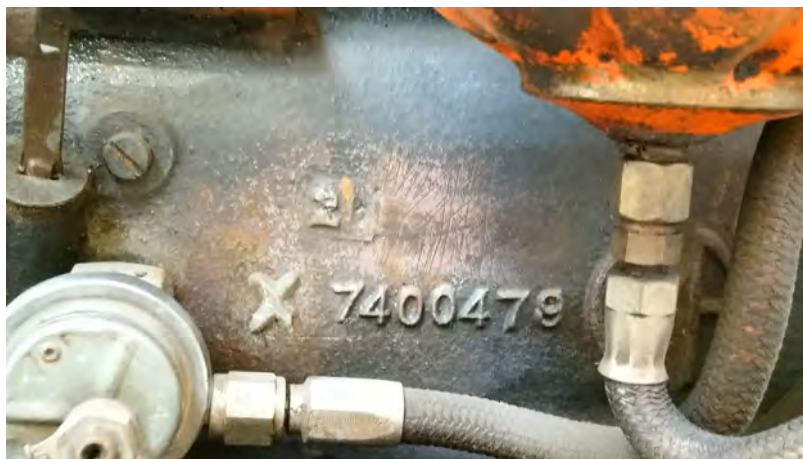
JP481 engine. Faked prototype engine. Note large X. This was made from body filler, you can also see where the cast GMH was ground off the block.
